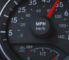
The color, illumination, legibility and even the type font and size of gauges is designed to deliver optimal viewing in varying light conditions, maximizing alertness and minimizing eye fatigue.
